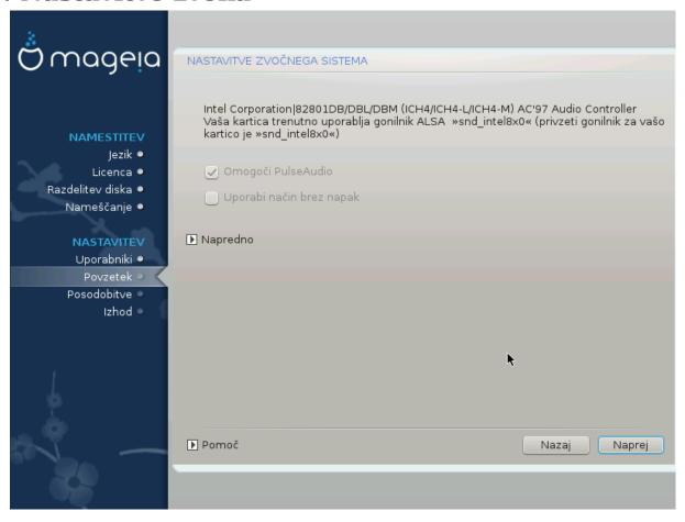
This screen shows the details of the sound card driver chosen for you by the installer, and this driver should work without problems.
