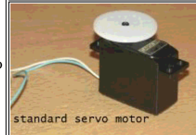
A standard servo modified to work as a motor. This is probably the best solution but we had this idea only after the robot was already built.
