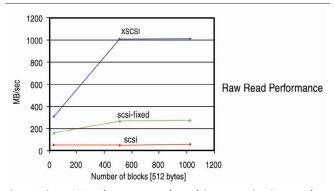
Figure 8. Linux XSCSI performance example: work-in-progress, interim example using 2.4.16 kernel; 120 processes reading from 120 disks (through driver only).
