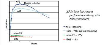
Figure 7. Filesystem performance comparison: AIM7 multi-user kernel workload, 2.4.17 kernel; 28 P Itanium prototype, 14GB, 120 disks; work-in-progress, interim example; varied filesystems only, but includes SGI enhancements and SGI-tuned kernel.
