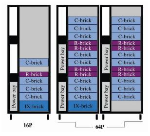
Figure 2. Two Possible NUMAflex Configurations
