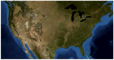
• "Imagery Topo" is a tile base map of orthoimagery in TNM as a backdrop, and a limited selection of topographic data (boundaries, names, transportation, contours, and hydrography).
