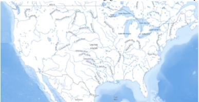
• "Shaded Relief" is a tile base map of terrain representation in the form of hillshades created from the 3D Elevation Program (3DEP). 3DEP maintains a seamless dataset of best available raster elevation data, in the form of digital elevation models (DEMs) for the conterminous United States, Alaska, Hawaii, and Territorial Islands of the United States.
