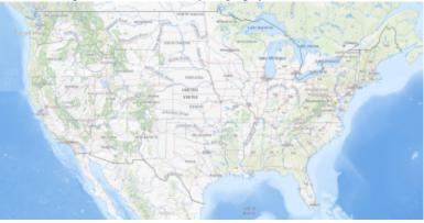
• "Imagery" is a tile base map of orthoimagery in TNM. Orthoimagery data typically are high resolution aerial images that combine the visual attributes of an aerial photograph with the spatial accuracy and reliability of a planimetric map. USGS digital orthoimage resolution may vary from 6 inches to 1 meter.
