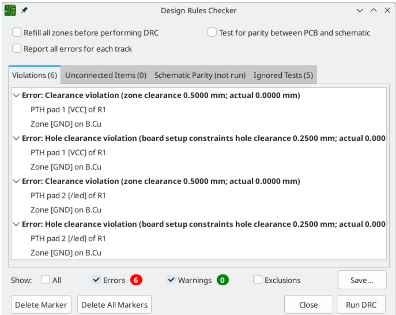
Close the DRC dialog, press **B** to refill the zone, and re-run DRC. Alternatively, check the **Refill all zones before performing DRC** checkbox and re-run DRC. All violations are fixed.
