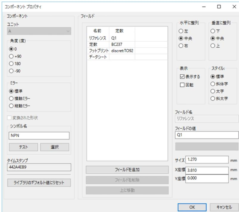
You can only use the properties dialog to edit one item at a time. To edit multiple items, use the Properties Manager, described below. There are also other tools that can be used to edit specific types of objects in bulk, such as the [Edit Text and Graphics tool](#) for editing text, labels, and graphic shapes, or the [Symbol Fields Table](#) for editing symbol fields in bulk.
