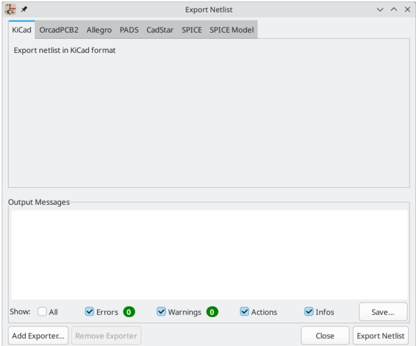
KiCad supports exporting netlists in several formats: KiCad, OrcadPCB2, Allegro, PADS, CADSTAR, Spice, and Spice Model. Each format can be selected by selecting the corresponding tab at the top of the window. Some netlist formats have additional options.
