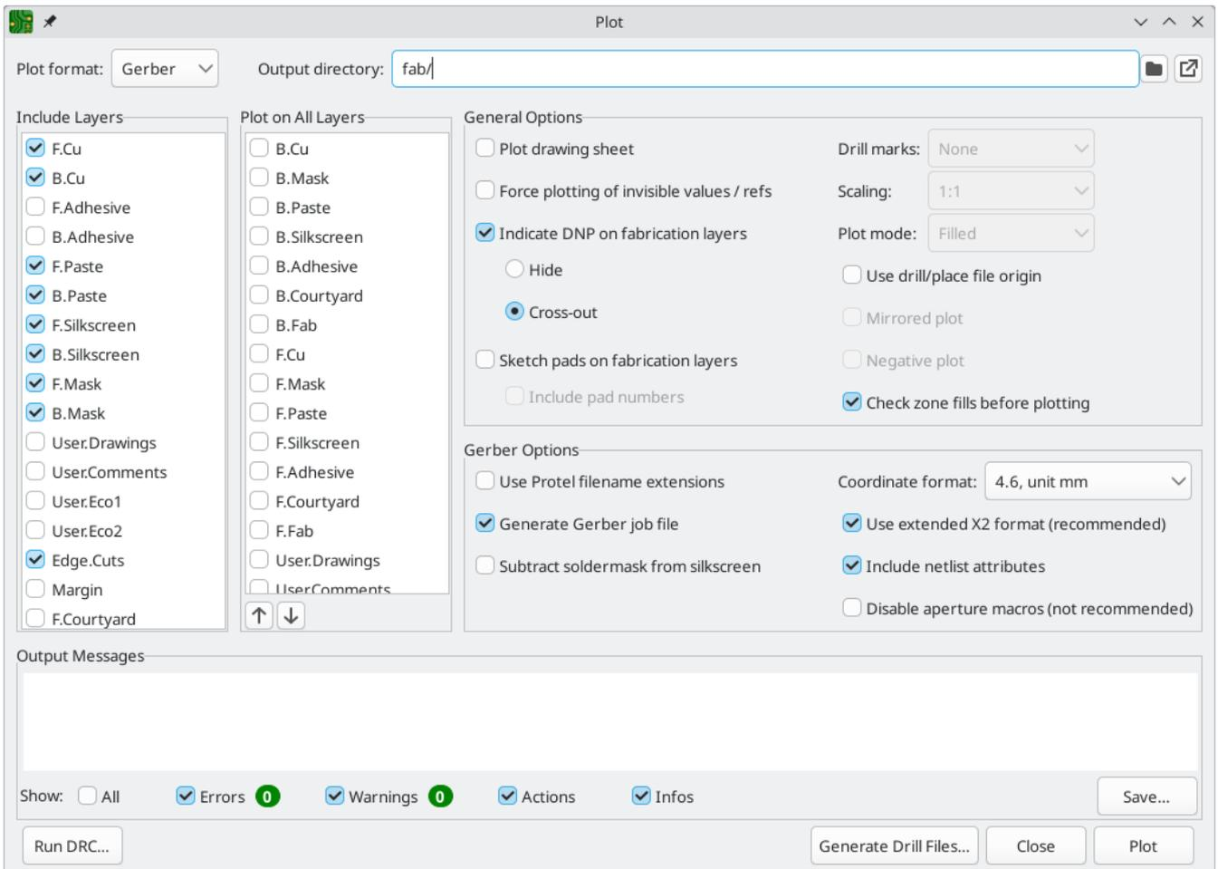
Click **Plot** to generate the Gerber files. Also click **Generate Drill Files...** and then **Generate Drill File** to create files specifying the location of all holes that will be drilled in the board. Finally, close the Plot dialog. The design is finished.
