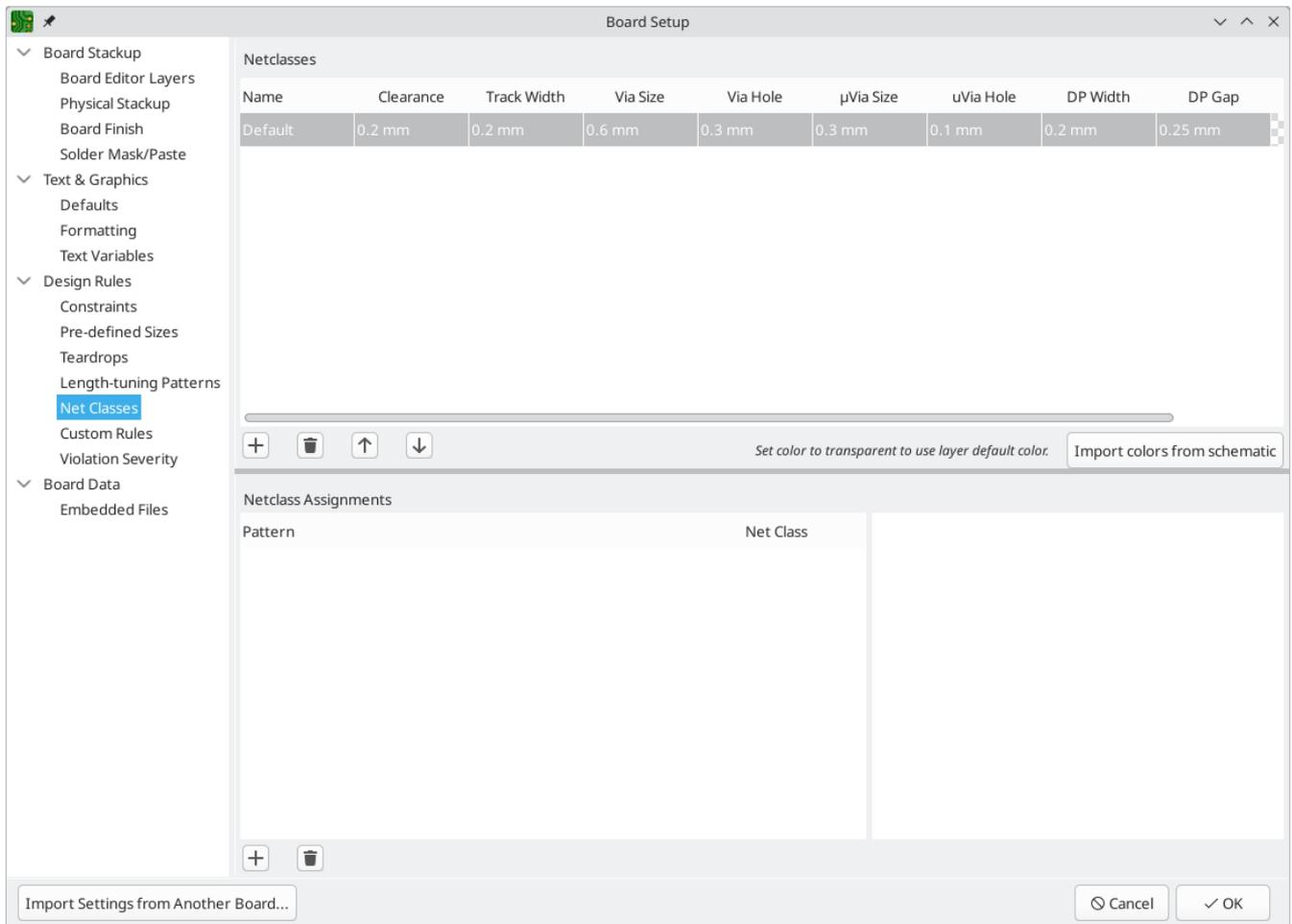
Track width and spacing can be managed manually by the designer during layout, but net classes are recommended because they provide an automatic way to manage and check design rules.
