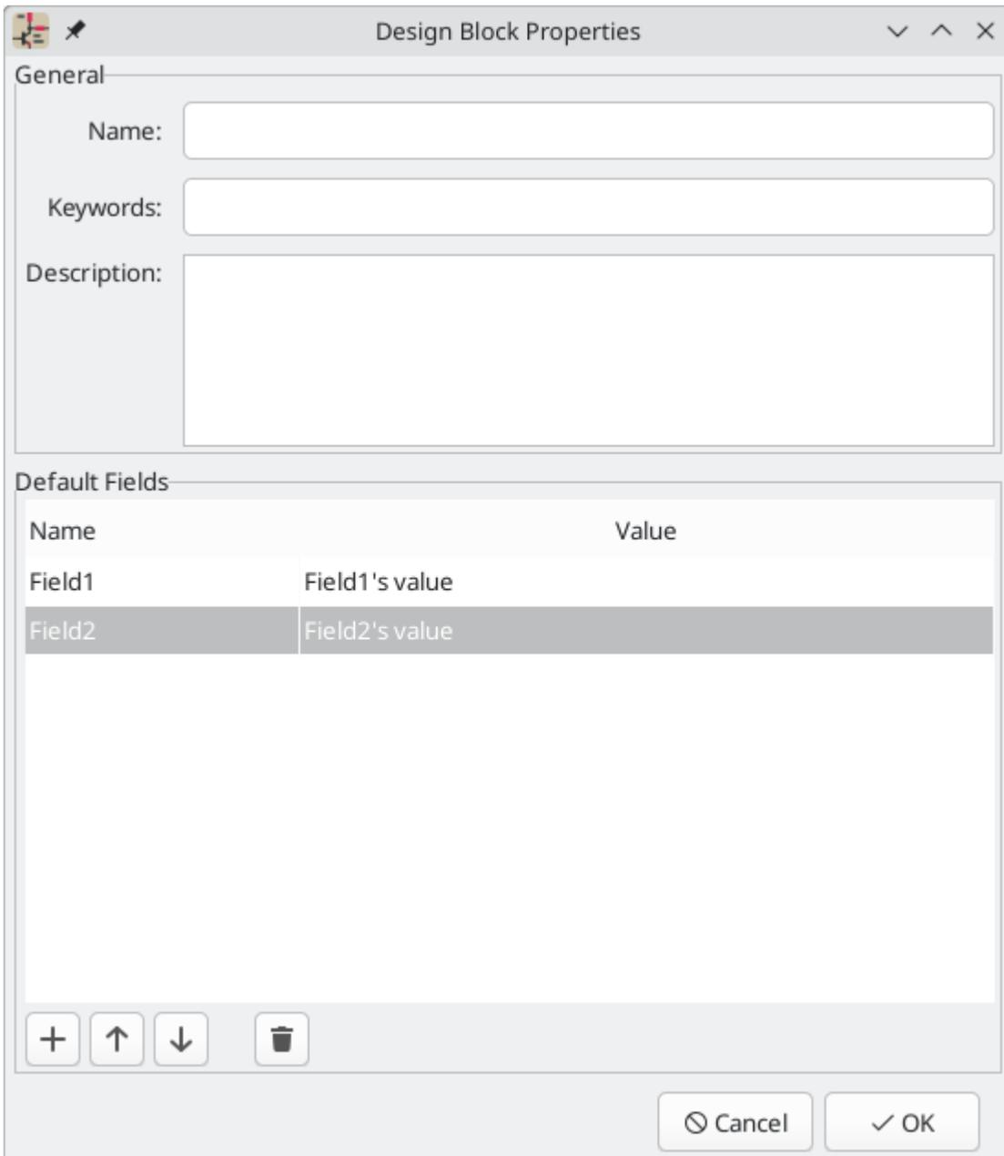
This brings up the Design Block Properties dialog, where you can edit the properties of the new design block.
