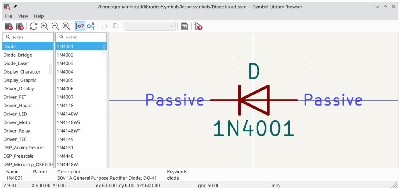
Double clicking the name of a symbol or using the
