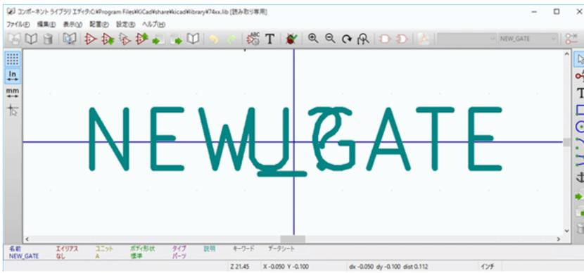
The blue cross in the center is the symbol anchor, which specifies the symbol origin i.e. the coordinates (0, 0). The anchor can be repositioned by selecting the
